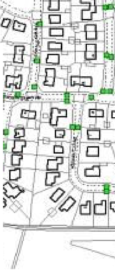
GIS record of freshly surveyed gully locations in West Garforth
